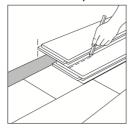
7. **Holes for pipes:** Measure the diameter of the pipe and drill a hole that is 20 mm larger. Saw off a piece as shown in the figure and lay the board in place on the floor. Then lay the sawed-off piece in place.
