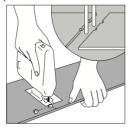
**8. Door molding and skirting:** Lay a board (with the decorative side down) next to the door molding and saw as shown in the figure. Then slide the floorboard under the molding.
